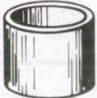
No. 7 P-234 Spacer 1/2" I.D. x 9/16" 1 Used.
